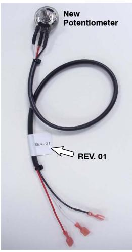
Connect the new potentiometer wire harness to machine wire harness wires as shown (white to 39/white, red to1B/red and black to13AA/black).
